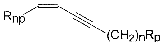
Figure 2. General structure of the analogues described in this work. Rnp= non-polar alkyl chain, Rp= polar alkyl chain.
